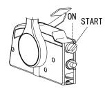
7. Immediately after the engine starts, release the main switch and allow it to return to "**ON**"(on).
