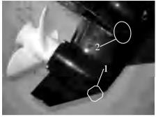
1.Gear oil drain screw
